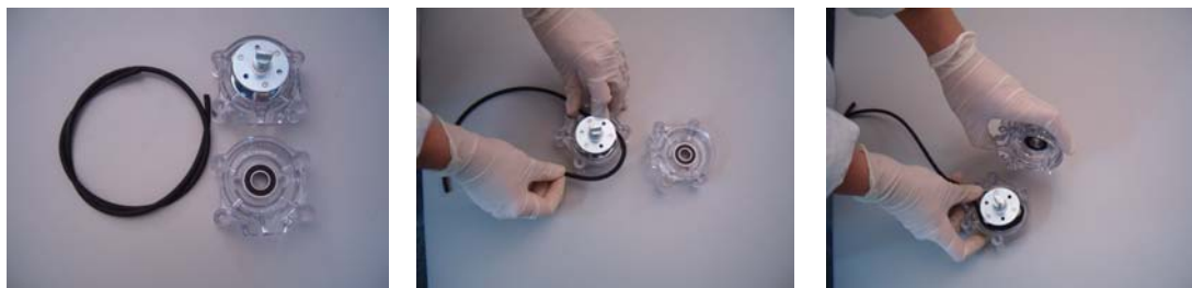
Figure 8-1: Pump tubing replacement details
